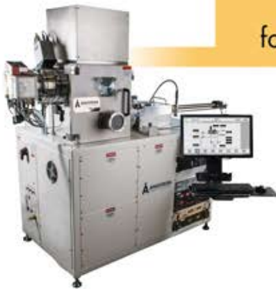
Cleanroom indium deposition system for sensor production
