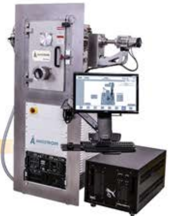
Cleanroom indium deposition system for sensor production
