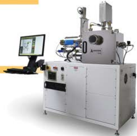
Dielectric optical sputtering system for broadband filters
