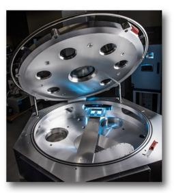
Substrate sizes up to 200mm x 200mm can be easily accommodated and the modules can be designed for use with larger substrates if desired. Throughput depends on process duration and complexity. However, the AERES software platform optimizes layer to layer transitions to reduce overall process time.
