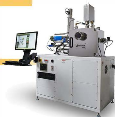
Dielectric optical sputtering system for broadband filters
